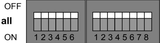
The dip-switches on the front panel are used to set E1 remote loop-back test and Ethernet port isolation functions.
