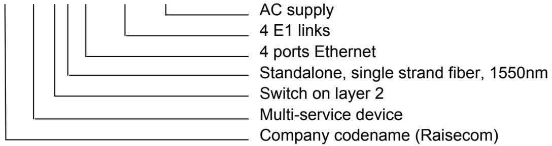
**Note:** Standalone single strand fiber Ethernet multiplexer: RCMS2504-240 should work with RCMS2304-240, viz. one RCMS2304-240 should connect with one RCMS2504-240.
